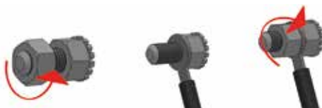
Figure 3. Connecting the unit to an electrical equalizing system
